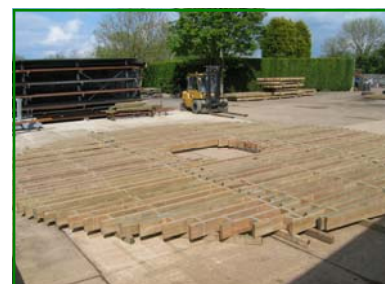
Factory check of pre-assembled timber matrix modules ready for loading onto delivery trans-
